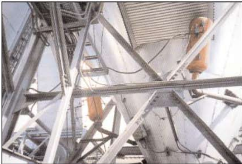
HIGH TEMPERATURE BIN: Recycling bin with 300°F temperature use ABS-4-10's. Long discharge pipes eliminate heat problem. Ask for Bulletin 9060.
